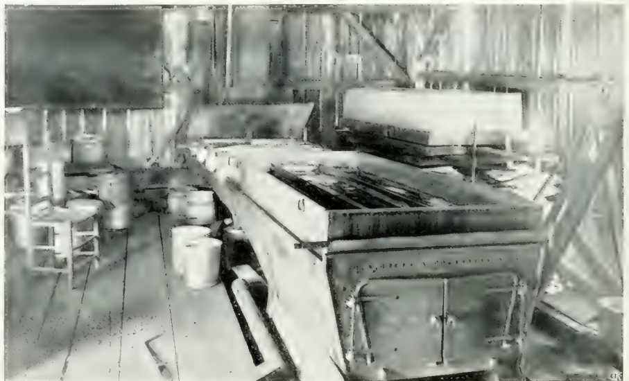
Evaporator in the sugar house. (Photograph supplied by Vermont Agr. Exp. Station.)
