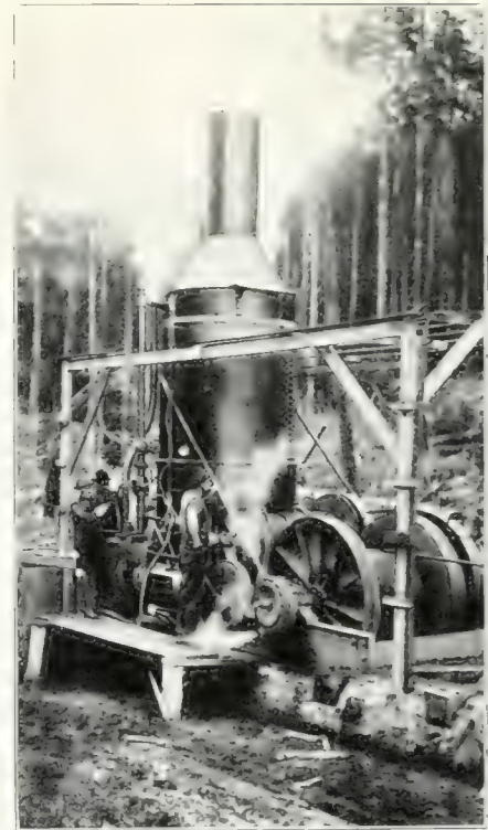
Heavy road engine at work on holdings of C. A. Smith Timber Co., Marshfield, Oregon.
