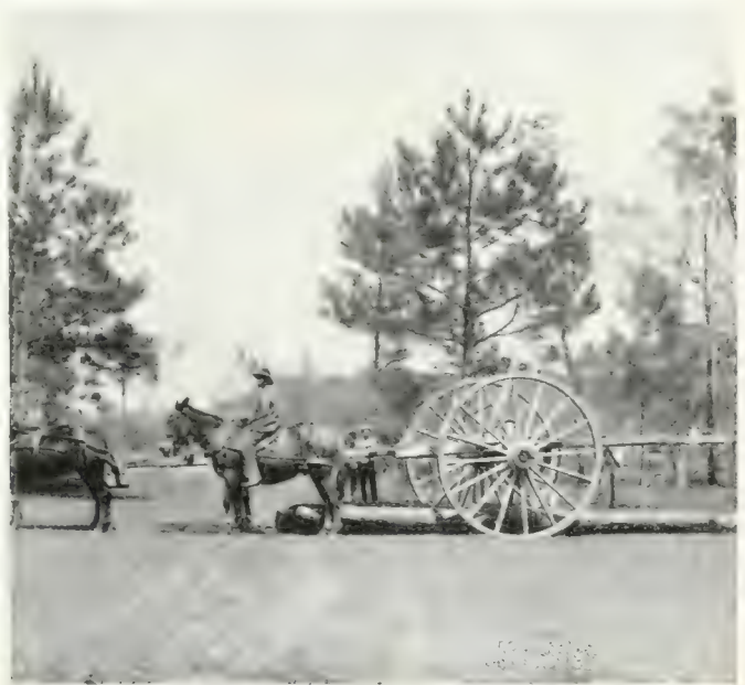
Logging by slip-tongue carts, side view, holdings of John L. Roper Lumber Co.
