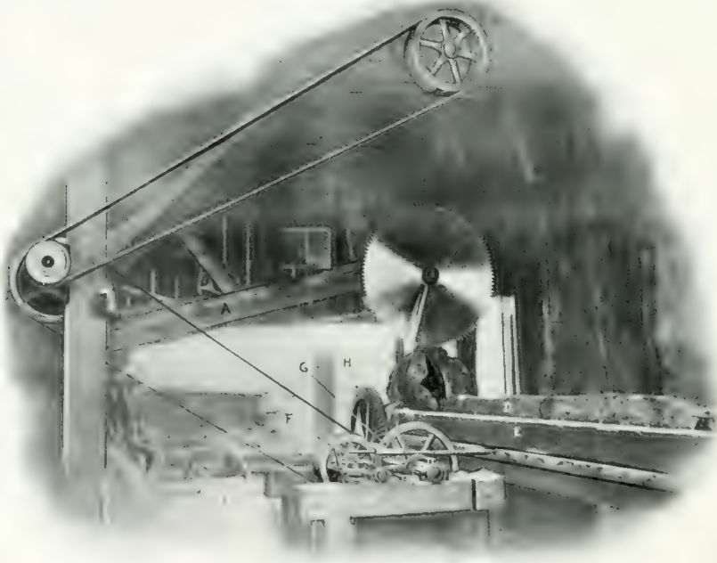
Overhead drop frame wood saw, made by M. Garland Co., Bay City, Mich. D is the log to be cut; C, the cut piece of wood; A is the drop saw frame; F, G, H, friction and geared log chain drive, which can be stopped at any desired point and started at will.
