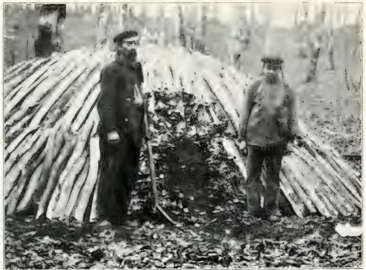
Small charcoal pit ready to receive a coating of beech mold and a covering of dirt, preparatory to charring.
