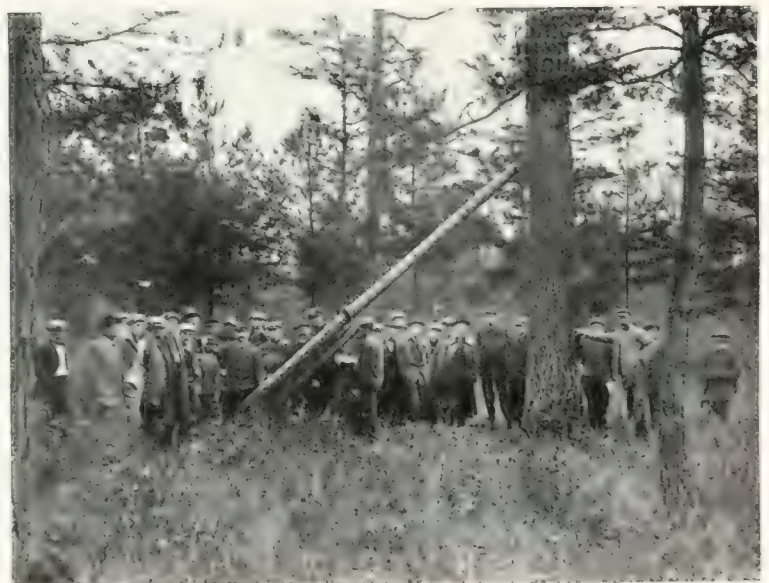
Felling an oak with roots and stump by the Buettner felling machine.
