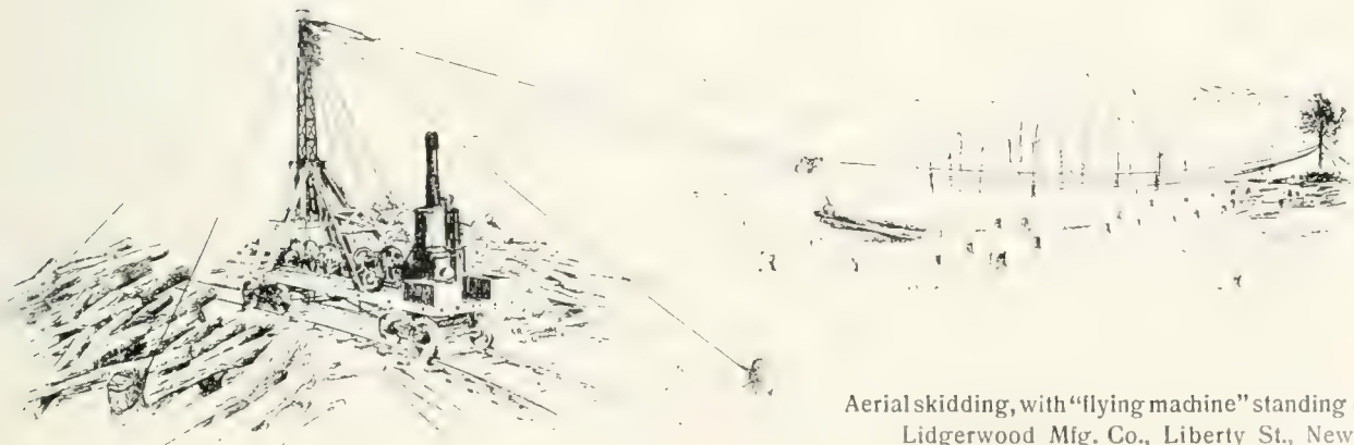
Arrangement of cables in aerial skidding, as devised by the Lidgerwood Mfg. Co.
