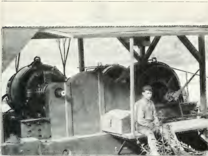
Westinghouse-Willamette electric skidder on trial at the C. A. Smith Mill, Marshfield, Oregon.
