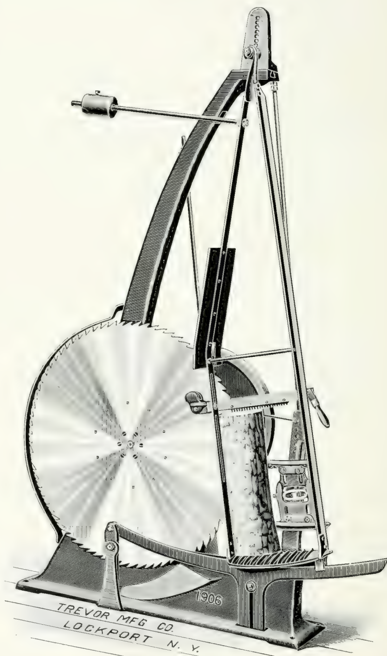
Heading sawing machine. Trevor Mfg. Co., Lockport, N. Y.
