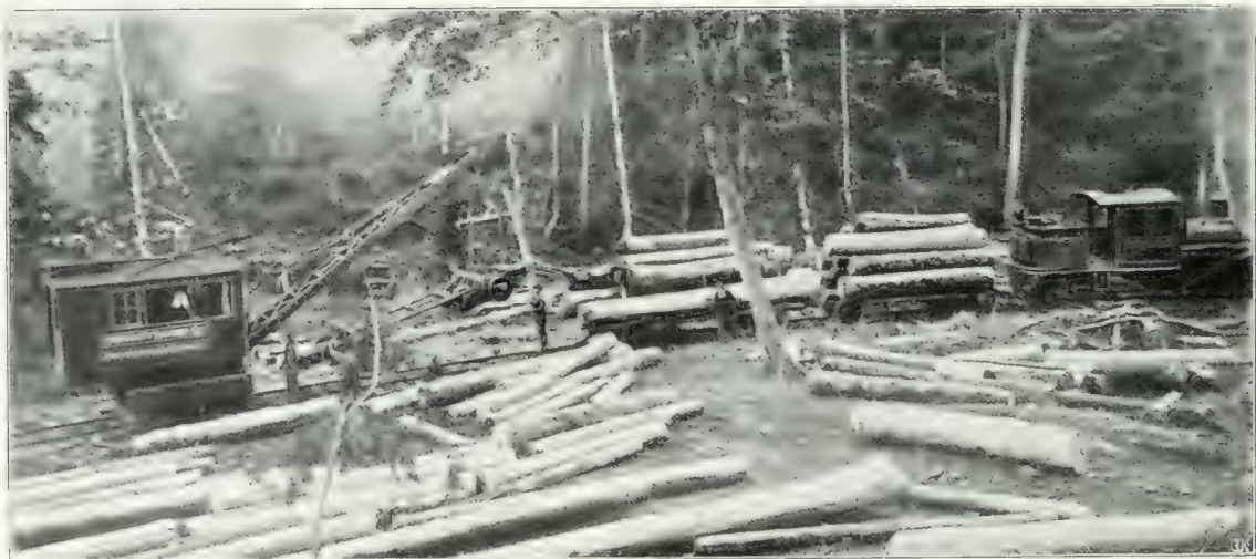
American log loader, self-propelling type, spotting its own empties by swinging them from the rear to the front.
