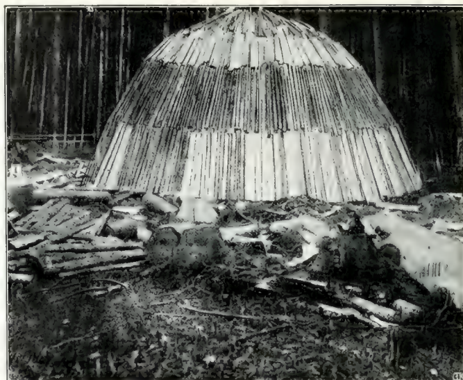
Large charcoal pit in Austria, ready to receive the covering.
