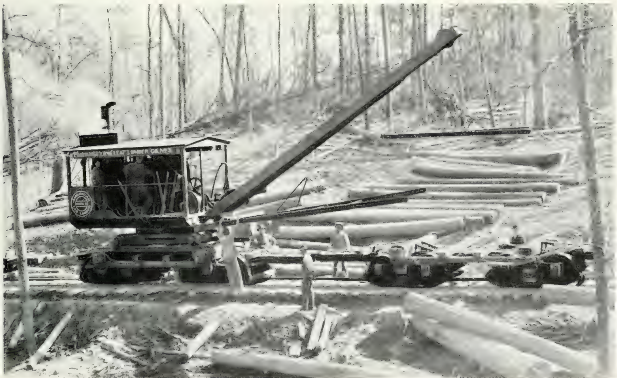
American log loader putting its own rail sections from one empty in front to another empty in the rear. American Hoist & Derrick Co., St. Paul, Minn.
