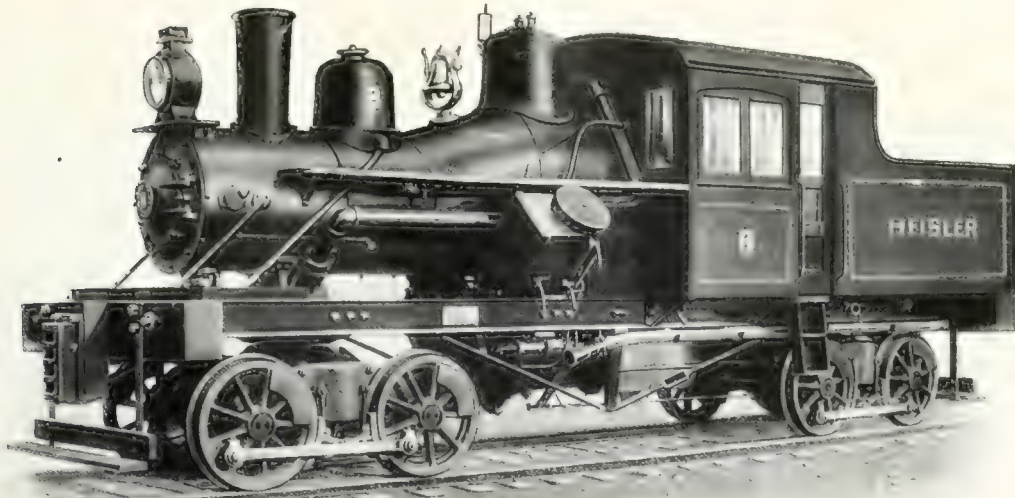
Side view of new type Heisler geared locomotive. Heisler Locomotive Works, Erie, Pa.
