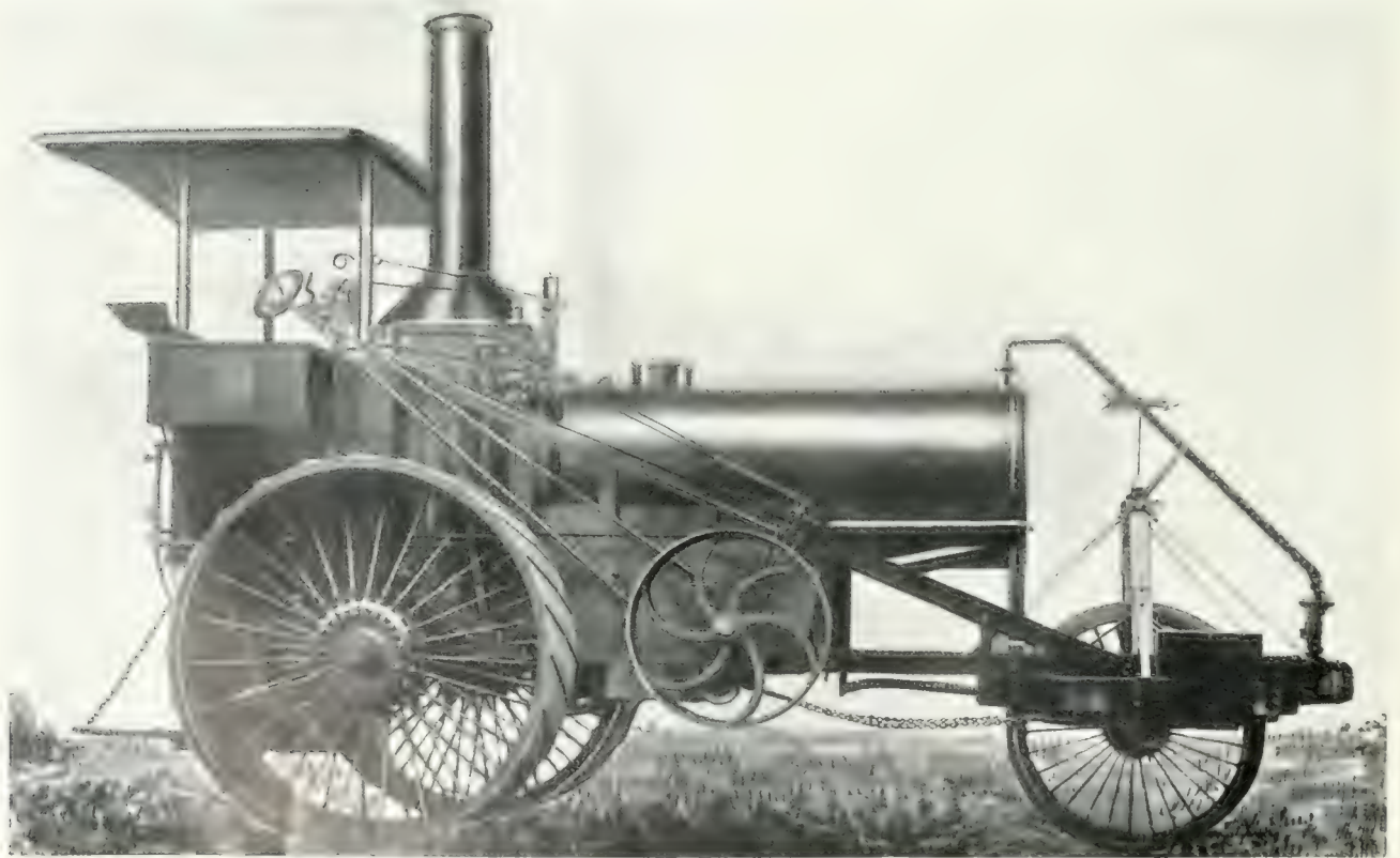
Three-wheel traction engine. Best Mfg. Co., San Leandro, Cal.
