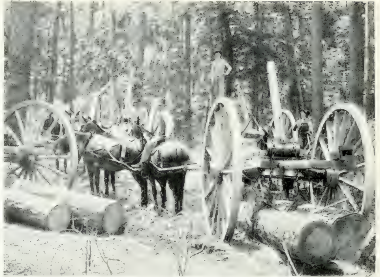
Skidding by two-wheelers. Photo by Clyde Iron Works, Duluth, Minn.
